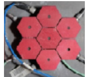
Seven hexagonal pads and load cells with cables.
